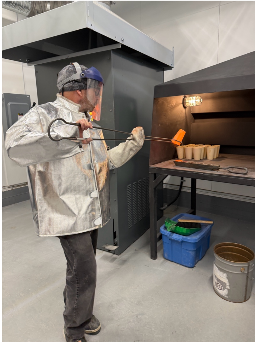
Samples being loaded into the furnace at the Company's newly commissioned fire assay laboratory near Smithers, B.C.
